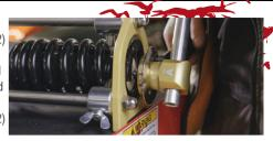
washer (Pos. 3). Max. torque for tightening is 25 Nm!
